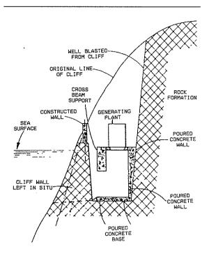
Figure 3: Norwegian OWC Plant
